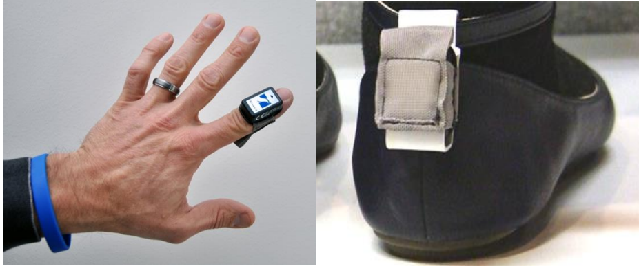
Figure 2: Kinesia Sensor Proper Positioning
